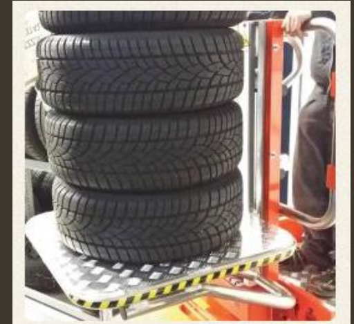
Ballast weights for polished or slippery floors
