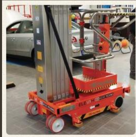
Ballast weights for polished or slippery floors
