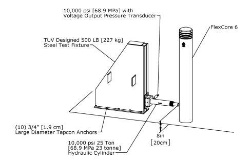
Products are tested for compliance to international standards and codes by taking dynamic measurements in real time of applied force and resulting deflection. Force and deflection measurements are used to determine the magnitude of energy transfer to the product by using principles of the work energy theorem. The criteria for product failure has been defined as a 4" [10 cm] deflection with the intent of balancing product robustness, floor space, and application for safe working conditions.
