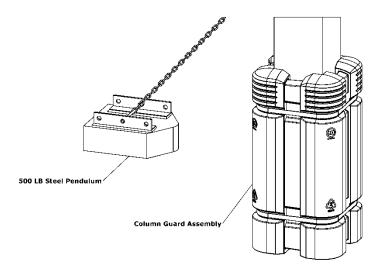
Column Guard was installed on a fabricated square vertical steel column and impacted with a 500-lb [227 kg] pendulum raised 1.8-ft [0.55 m] from the point of impact to provide an impact energy of 900 ft-lbs. [1222.5 Nm] This impact is equivalent to a 6500 lb [2948 kg] vehicle traveling at 2 mph [3.3 km/h].
